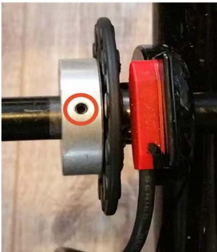
Image 4: Allen screw next to disc magnet.
