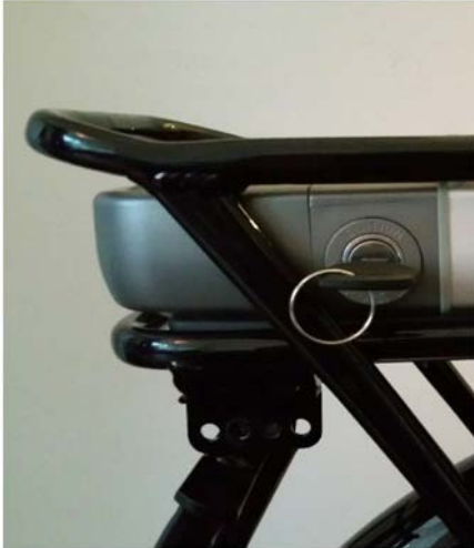
Image 9: Key horizontal, battery is on.
