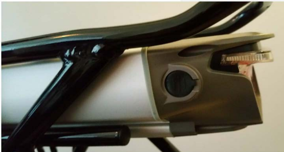
Image 12: Charge socket, pull the tab.
