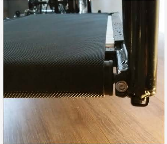
Image 8: Tension adjustment bolt, right.
