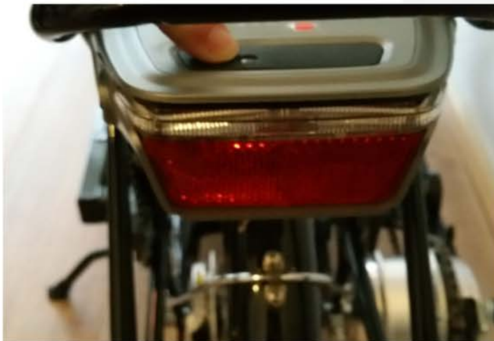
Image 22: Rear light, button on the battery.
