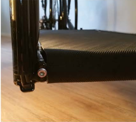
Image 7: Tension adjustment bolt, left.
