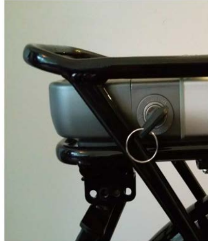
Image 10: Key vertical, battery is off.
